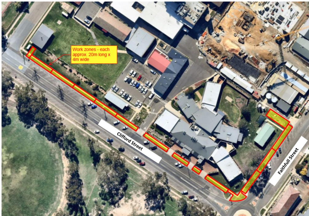
Image 1: Works location and work section plan.
