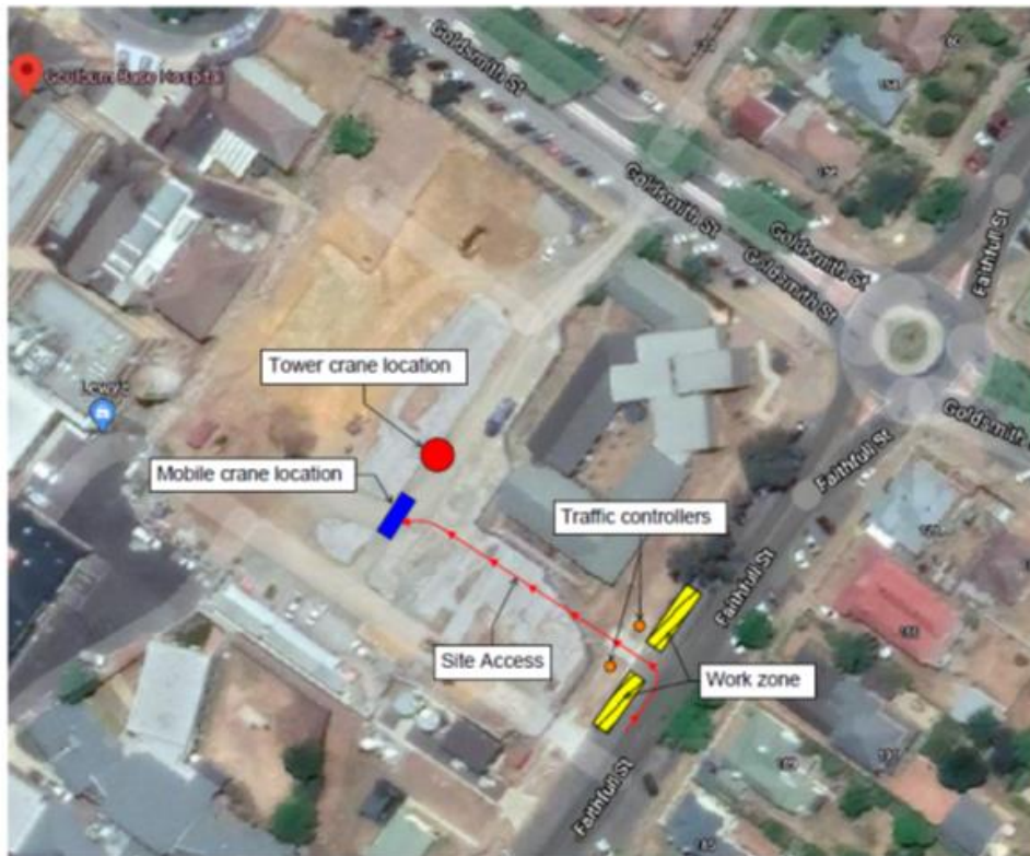
Tower crane establishment - Set up plan
